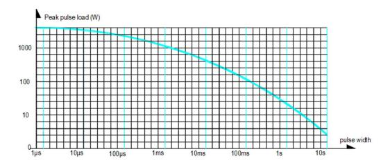
Wire wound resistor is capable of quite high pulse loading with the peak pulse load power curve shown in the draft.
